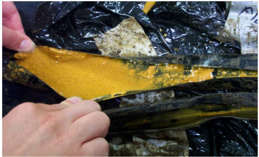
Figure 4. Chemical precipitation in an SDI dripline.
