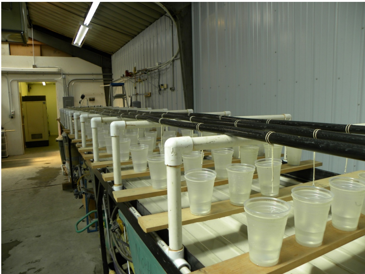
Figure 6. Laboratory bench arrangement for measuring emitter discharge from 30 contiguous emitters.
