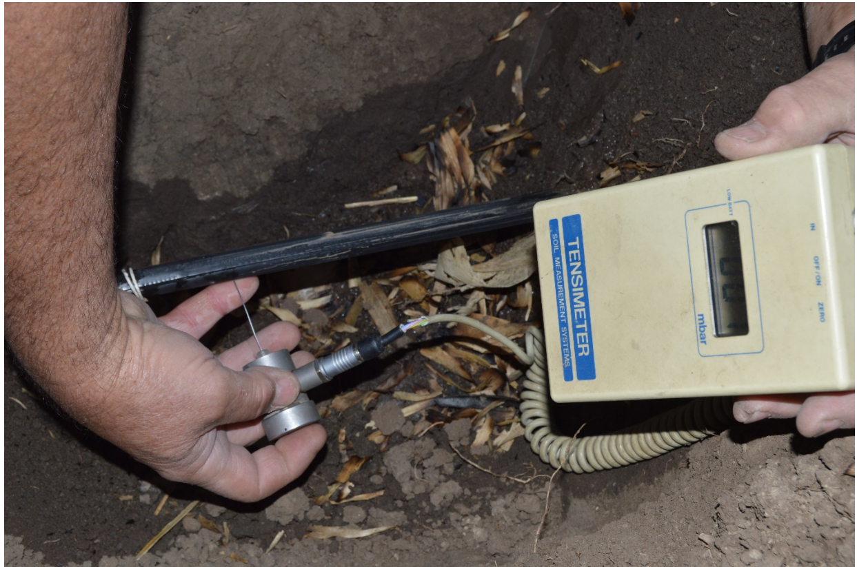
Figure 3. Measuring dripline pressure at the emitter by puncturing the dripline with a needle tube attached to a pressure transducer.
