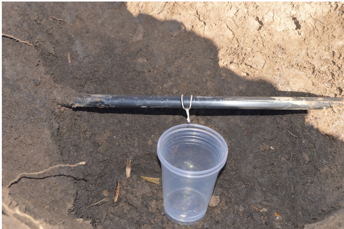
Figure 2. Arrangement for measuring emitter discharge over a 20 minute period.
