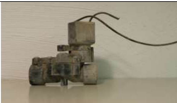
Figure 12. A broken solenoid wire on a zone valve might go unobserved if producers do not monitor there system flowrate and pressure.
