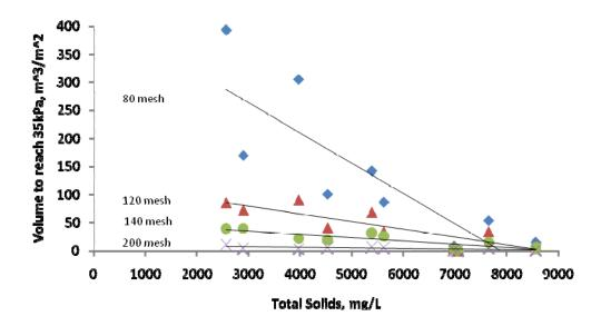
Figure 2. Volume of biological effluent from beef or swine lagoons passing through a disk filter before the pressure differential reaches 35 kPa (5 psi). The mesh sizes are 80 mesh (openings of 200 um), 140 mesh (openings of 130 um), 120 mesh (openings of 115 um), and 200 mesh (openings of 55 um). Each point shown is the average of four replicates. The volume shown is the volume of effluent per area of the filter (unpublished data, Trooien and Lamm, 1999).
