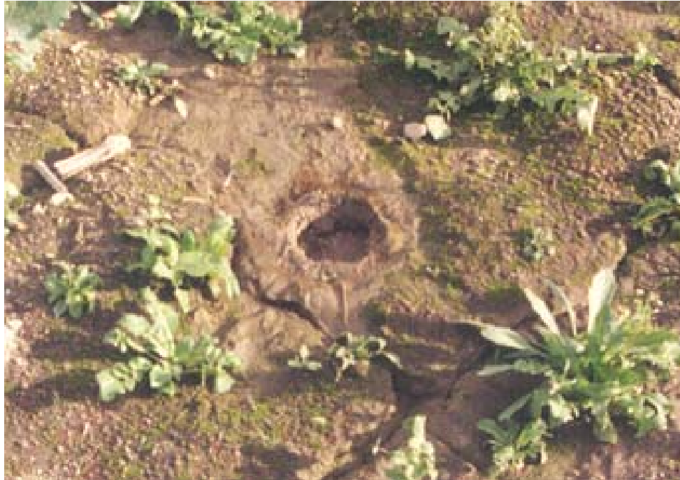
Figure 3. Caldera resulting from surfacing of water from an SDI emitter in California. Photo courtesy of F. R. Lamm, Kansas State University.
