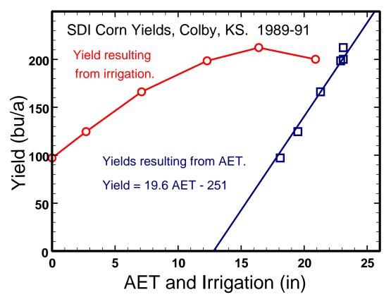
Figure 2. Corn yield as related to irrigation and calculated evapotranspiration (AET) in a SDI water requirement study, Colby, Kansas, 1989-1991.
