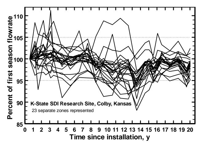
Figure 15. Stability in zone flowrates from the initial first season as related to time for an SDI system installed at Kansas State University, Colby, Kansas, 1989-2009.
