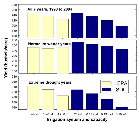
Figure 11. Variation in corn yields across years and weather conditions as affected by irrigation system type and capacity, Colby Kansas.
