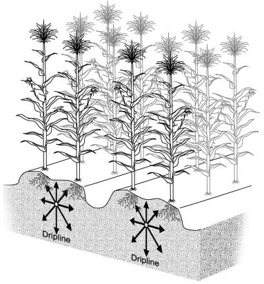
Figure 1. Physical arrangement of the subsurface dripline in relation to the corn rows.
