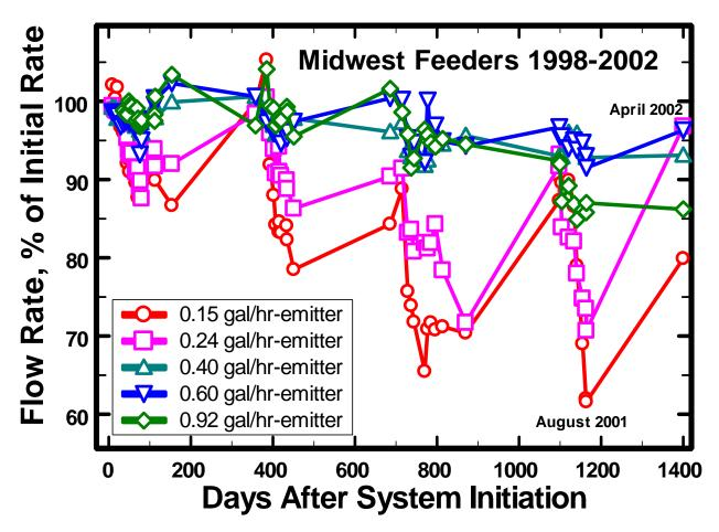
Figure 13. Decrease in emitter discharge during four seasons of operation of an SDI system with biological effluent at Midwest Feeders, Ingalls, Kansas, 1998 to 2002.
