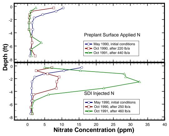
Figure 9. Nitrate concentrations in the soil profile for preplant surface-applied and SDI injected nitrogen treatments, Colby, Kansas, 1990-91. Data is for selected nitrogen fertilizer rate treatments with full irrigation (100% of AET).
