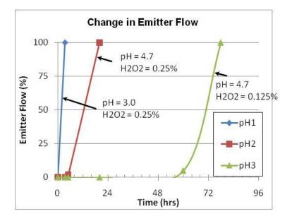
Figure 7. Relative emitter flow over time of clogged emitters treated with 0.25%  $H_2O_2$  at pH 3, 0.25%  $H_2O_2$  at pH 4.7, and 0.5%  $H_2O_2$  at pH 4.7 solutions with pressure at 30 psi.
