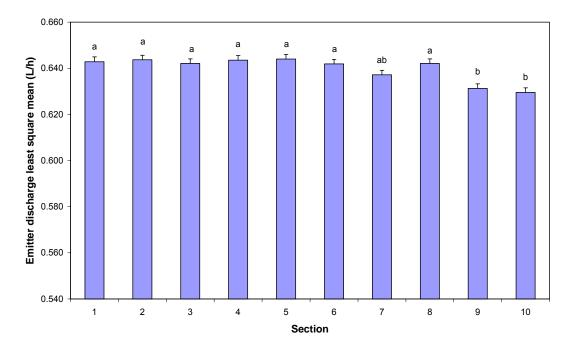
Figure 6. Discharge from the SDI emitters (least square mean ± standard error) as affected by section of the dripline (Section 1 is the inlet and Section 10 is the distal end). Different lowercase letters above each column indicate significant differences at P<0.05. This data is averaged across all flushing treatments to indicate the effect of location within the dripline on emitter clogging.
