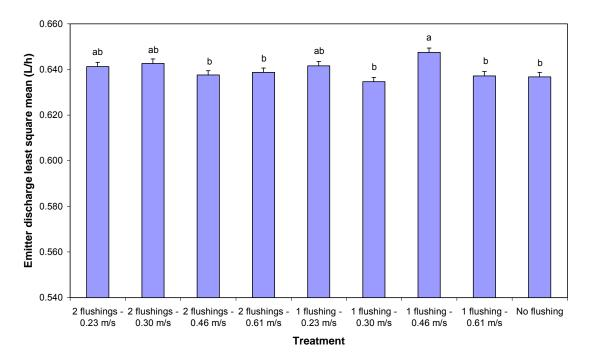
Figure 5. Discharge from the SDI emitters (least square mean ± standard error) as affected by flushing frequency and flushing velocity. Different lowercase letters above each column indicate significant differences at P<0.05. This data is averaged across all dripline sections to represent the overall effect on the dripline of flushing treatment.
