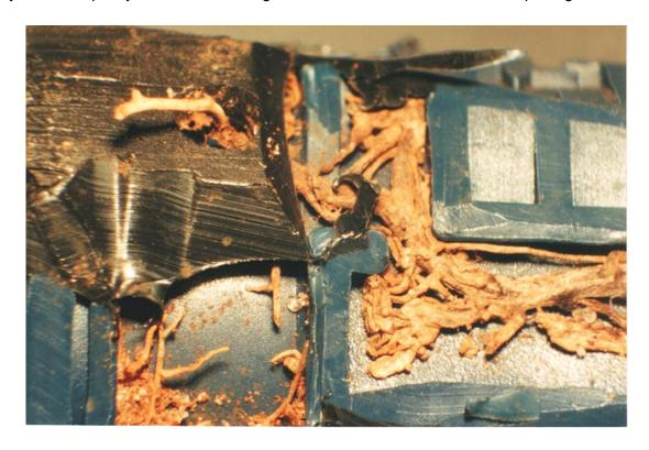
Figure 6. Single coffee plant root entering an emitter can enlarge into a large root mass once inside the emitter and dripline. Photo courtesy of Rubens Duarte Coelho, University of Sao Paulo, ESALQ / Brazil.
