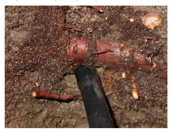
Figure 7. Subsurface dripline pinched by peach tree root in California, USA. Photo courtesy of T. Trout, USDA-ARS, Parlier, California.
