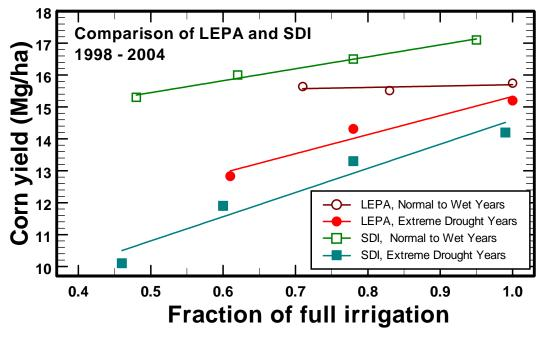
Figure 5. Corn grain yield as affected by irrigation system type (LEPA sprinkler and SDI) for various irrigation regimes in normal to wetter years and extreme drought years, KSU Northwest Research-Extension Center, Colby, Kansas.
