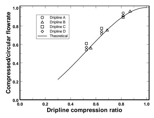
Figure 2. Decrease in flowrate resulting from deforming a circular cross-section into an elliptical cross-section. The dripline compression ratio is equal to the minor axis of the elliptical (compressed) dripline divided by the original circular dripline diameter. The solid line represents the theoretical relationship, and the data points are for the four driplines tested. After Hills et al. (1989).
