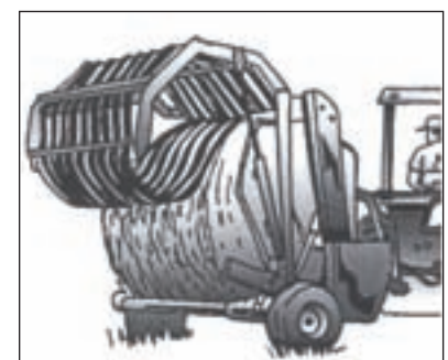
Figure 2. Be sure no one is near the rear gate when it is being raised or lowered.
