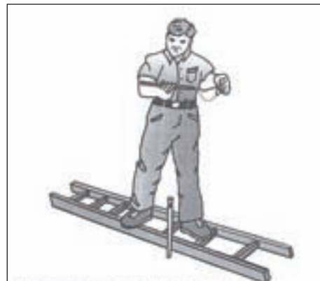
Figure 2. Proper procedure for monitoring hay temperatures.
