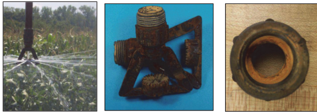
Figure 4. Nozzle incrustation for center pivot SN 7-18-99.
