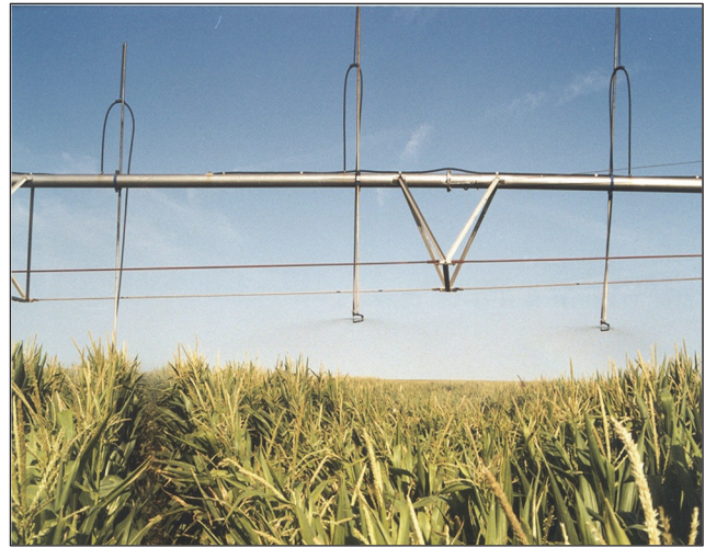
Figure 14. Irregular performance of in-canopy and near-canopy sprinkler-irrigated corn near Colby, Kansas, during extreme drought year of 2002. Nozzle on the left is within the canopy and not visible.
