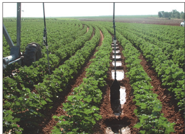
Figure 4. LEPA irrigation of cotton, at the Texas A&M AgriLife Research Center, Halfway, Texas.
