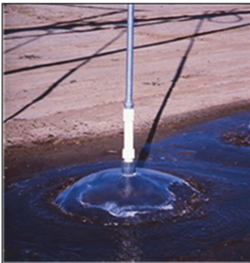
Figure 2. Irrigation applicator developed, built, and installed on initial LEPA pivot conversions. Orifice sizes were machined in 0.4 mm increments and placed appropriately to accommodate uniform water distribution along the pivot lateral at the Texas A&M AgriLife Research Center, Halfway, Texas, in 1979.
