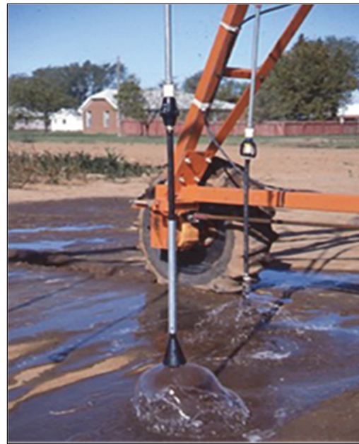
Figure 3. Prototype LEPA applicator manufactured by Rainbird in the early 1980s.
