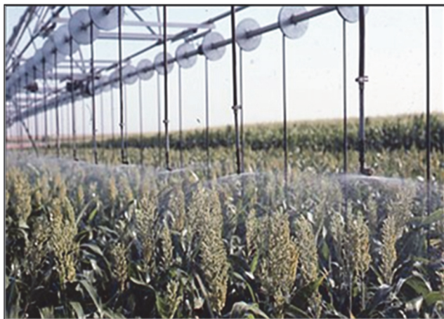
Figure 5. Multifunction irrigation and chemigation system (MFIS) applying low-volume solution to grain sorghum canopy. Auxiliary chemical nozzles automatically turned on and off while oscillating over a preset range as the MFIS moved through a field at the Texas A&M AgriLife Research Center, Halfway, Texas.
