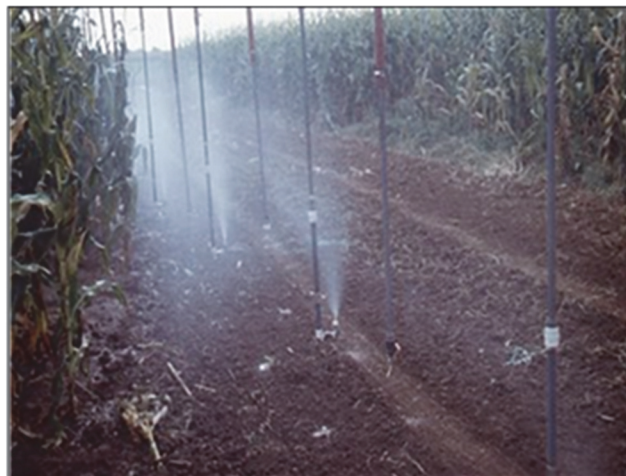
Figure 6. Stationary in-canopy chemigation nozzles on LEPA style drops at the Texas A&M AgriLife Research Center, Halfway, Texas.
