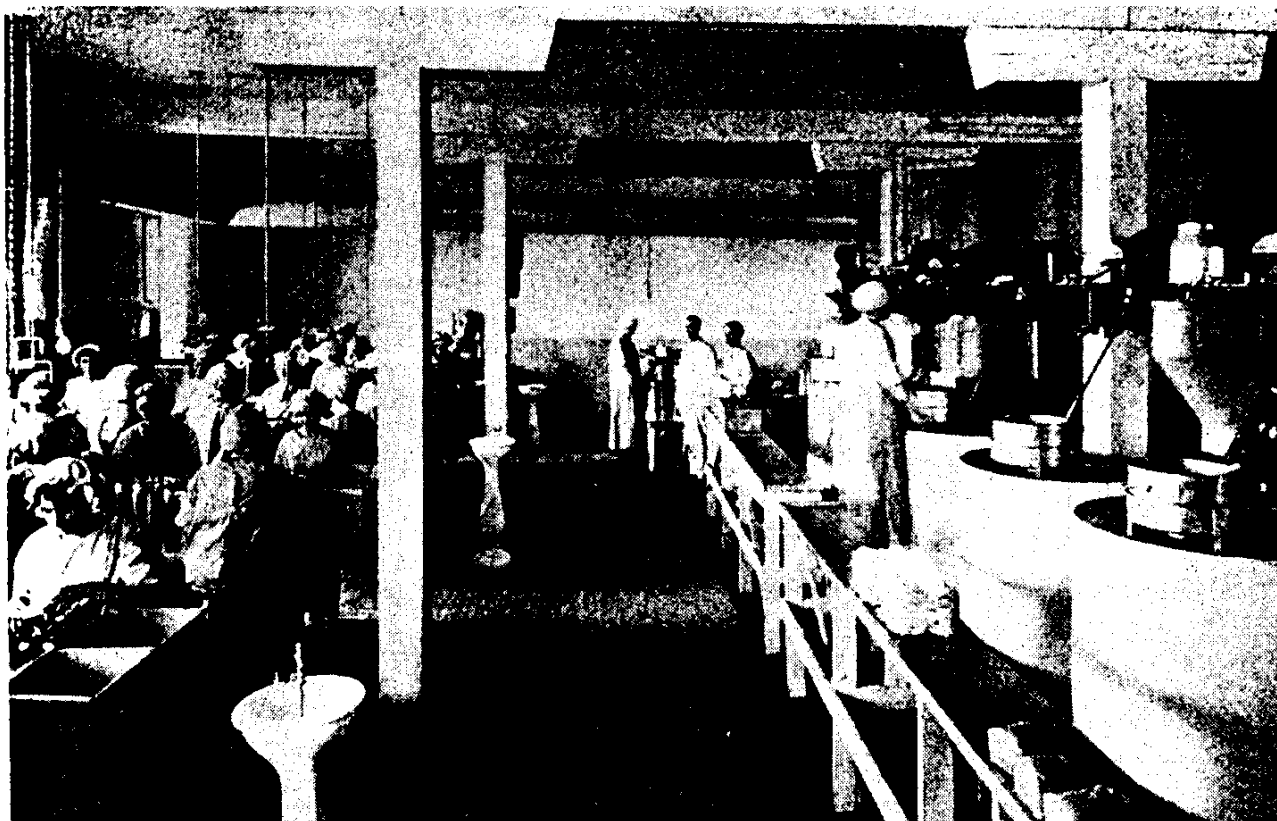
FIG. 2. The egg-breaking room of Figure 1 as it appeared in 1912 after recommendations of the Food Research Laboratory, U. S. Department of Agriculture, to improve sanitation and technology had been adopted.
