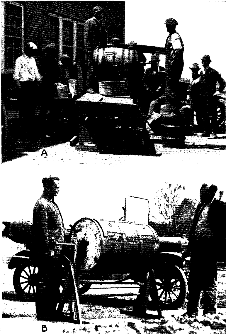
FIG. 13.—Homemade barrel treaters. (A) Wooden barrel mounted on platform. (B) Oil drum made into dust treater.
