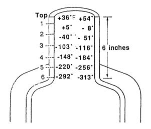
Figure 2. The drawing illustrates the temperature variation in the neck of the nitrogen refrigerator. Keep goblet at least two inches from the top when selecting straw.
