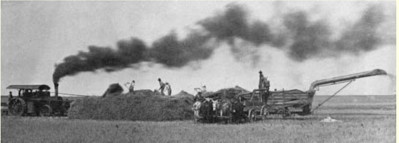
Threshing headed wheat using Reeves engine and Avery separator, from the stack, September 1912.
