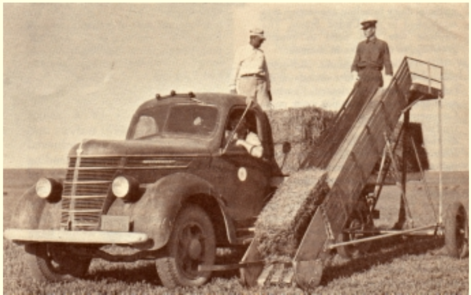
Automatic hay-bale pickup and loader designed and built at Fort Hays Station, 1946. (About the same time the Station designed and built a self-propelled field silage cutter that reduced cost of putting up silage 62 percent.)
