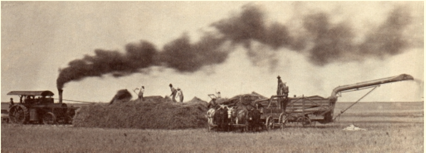
Threshing headed wheat using Reeves engine and Avery separator, from the stack, September 1912.
