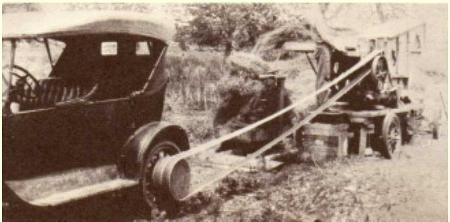
Threshing flax near Thayer, in the early 1920s, using Model T to provide belt power for thresher.
