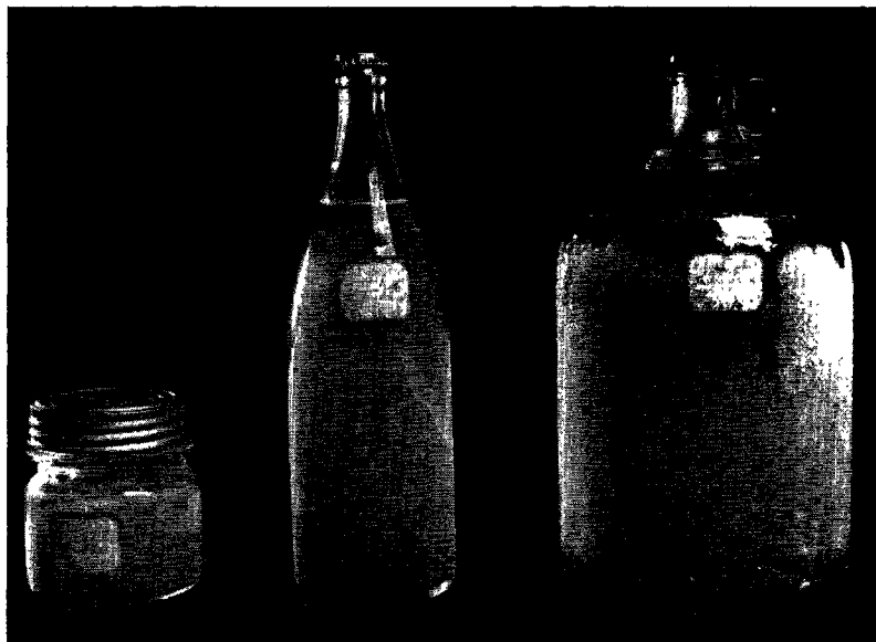
FIG. 2.—Containers used in storing fruit juices in frozen food lockers. (1) Wide-mouthed fruit jar with a small shoulder. (2) Bottle which tapers too much. Should be filled to a point below the label. Before freezing this bottle was filled to the top of the label. Note the amount of expansion. (3) Glass jug. Before freezing this jug was filled to top of label. Note the amount of expansion of apple juice.
