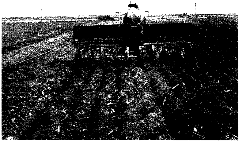
FIG. 9.—Drilling Wheatland with a 14-inch deep-furrow drill.
