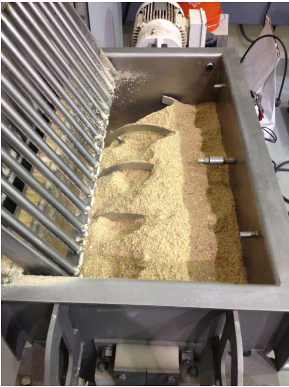
Figure 2. The 60-lb double-ribbon mixer with the corn-soybean meal-based diet. The ribbons are visible when the mixer is filled to capacity.
