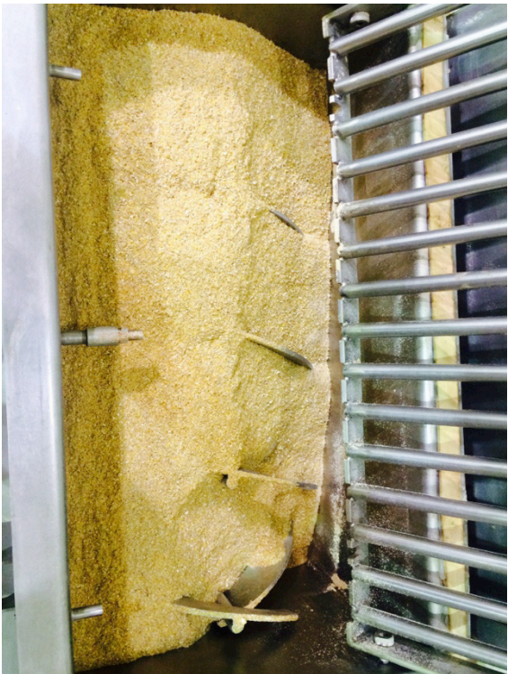
Figure 3. The 60-lb double-ribbon mixer with the low-bulk-density ingredients. Unlike the corn-soybean meal-based diet, the ribbons are less visible, illustrating the extra volume that the low-bulk-density diet consumes in the mixer.
