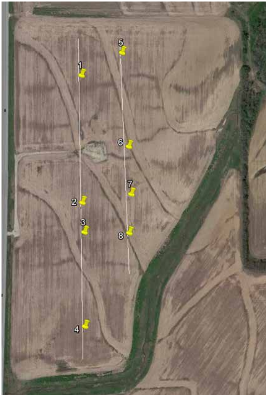
Figure 1. Sampling protocol for on-farm determination of yield-limiting factors for crop production. Sampling protocol for on-farm determination of yield-limiting factors in production fields showing transects (white lines) through the field with sampling positions 1 through 8. Detailed measurements of soil and crop parameters were taken from within 3 ft 2 at each sampling position. Combine harvest of 100 ft of row was measured around each sampling position for total yield, seed size, and quality. Wet conditions during harvest prevented machine-harvested sampling of soybean.
