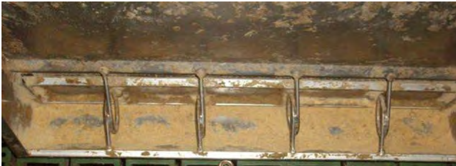
Figure 8. Narrow feeder adjustment with 70% pellets + 30% fines (minimum feeder gap was 0.50 in. with a maximum gap of 0.75 in.) averaged 61% feeder pan coverage.
