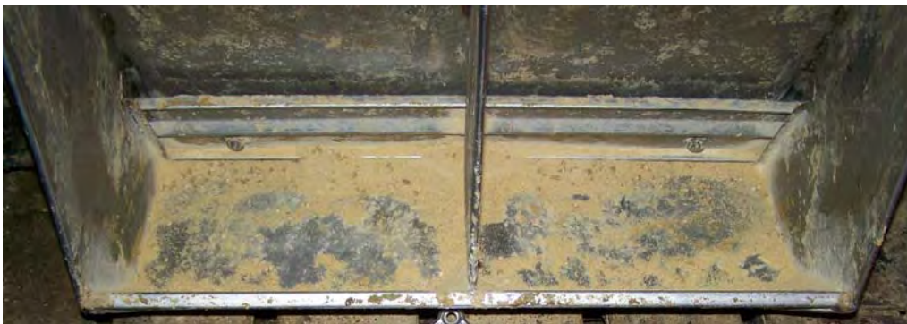
Figure 2. Phase 1 narrow feeder adjustment with 50% pellets and 50% fines (minimum feeder gap was 0.5 in. with a maximum gap of 0.75 in.) averaged 49% feeder pan coverage.
