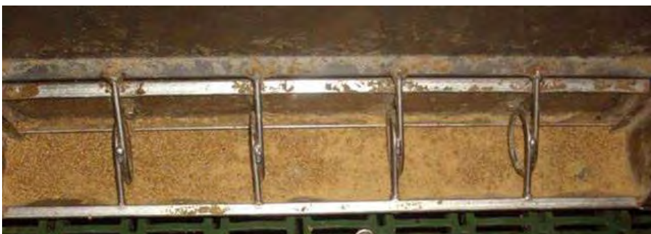
Figure 12. Wide feeder adjustment with screened pellets (minimum feeder gap was 1.00 in. with a maximum gap of 1.25 in.) averaged 97% feeder pan coverage.
