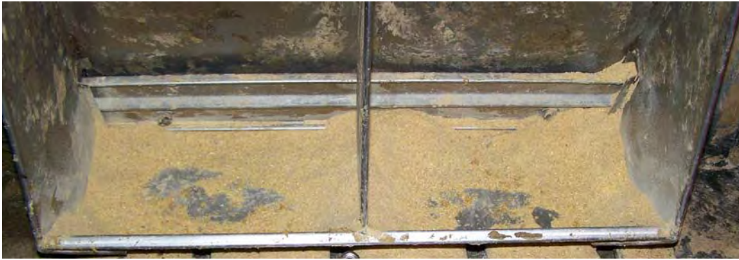
Figure 10. Phase 2 wide feeder adjustment with meal diet (minimum feeder gap was 1.00 in. with a maximum gap of 1.25 in.) averaged 90% feeder pan coverage.
