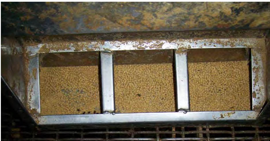
Figure 6. Wide feeder adjustment with screened pellets (minimum feeder gap was 1.00 in. with a maximum gap of 1.25 in.) averaged 93% feeder pan coverage.
