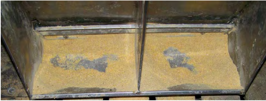
Figure 13. Phase 3 narrow feeder adjustment with meal diet (minimum feeder gap was 0.5 in. with a maximum gap of 0.75 in.) averaged 89% feeder pan coverage.
