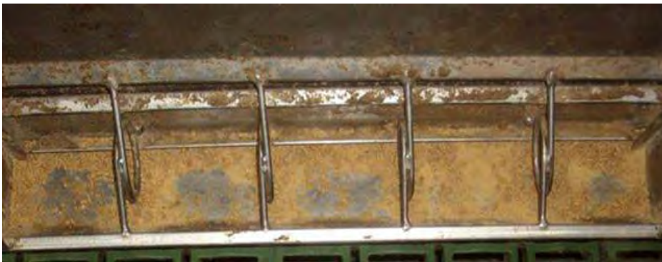
Figure 9. Narrow feeder adjustment with screened pellets (minimum feeder gap was 0.50 in. with a maximum gap of 0.75 in.) averaged 57% feeder pan coverage.
