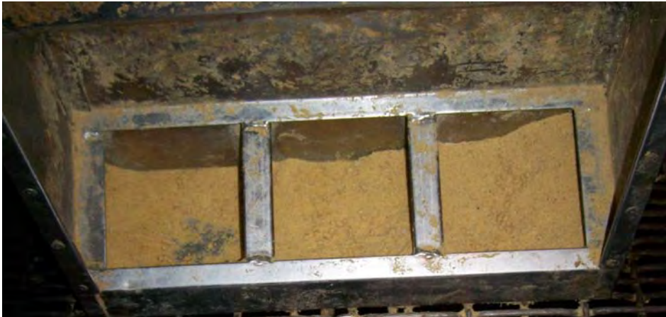
Figure 5. Wide feeder adjustment with 70% pellets + 30% fines (minimum feeder gap was 1.00 in. with a maximum gap of 1.25 in.) averaged 98% feeder pan coverage.
