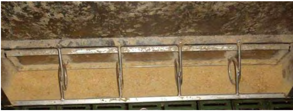
Figure 10. Wide feeder adjustment with meal diet (minimum feeder gap was 1.00 in. with a maximum gap of 1.25 in.) averaged 98% feeder pan coverage.
