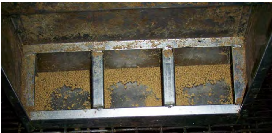
Figure 3. Narrow feeder adjustment with screened pellets (minimum feeder gap was 0.50 in. with a maximum gap of 0.75 in.) averaged 37% feeder pan coverage.
