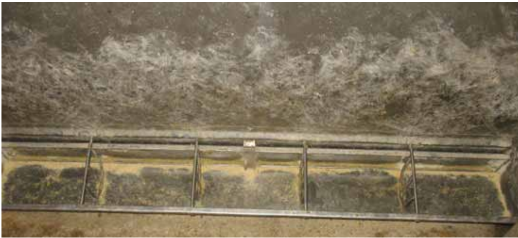
Figure 4. Conventional dry feeder at setting 6 with a 0.59- to 0.81-in. opening and \approx 9% pan coverage.
