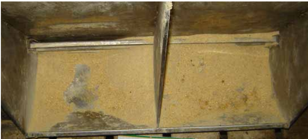
Figure 3. Wide feeder adjustment (minimum feeder gap was 1.00 in. with a maximum gap of 1.25 in.) averaged 75% feeder pan coverage.
