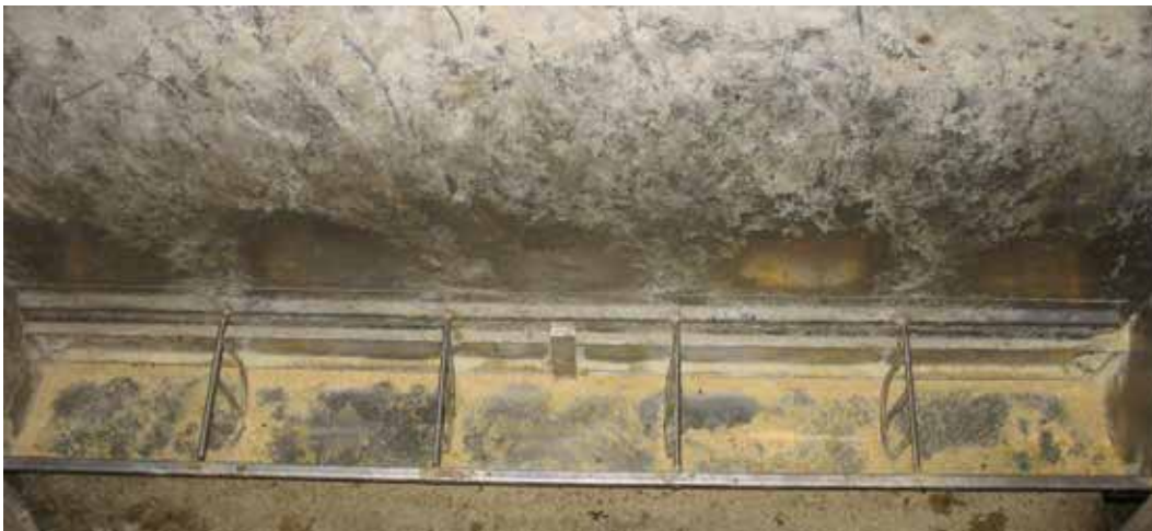
Figure 8. Conventional dry feeder at setting 6 with a 0.58- to 0.82-in. opening and \approx 27% pan coverage.
