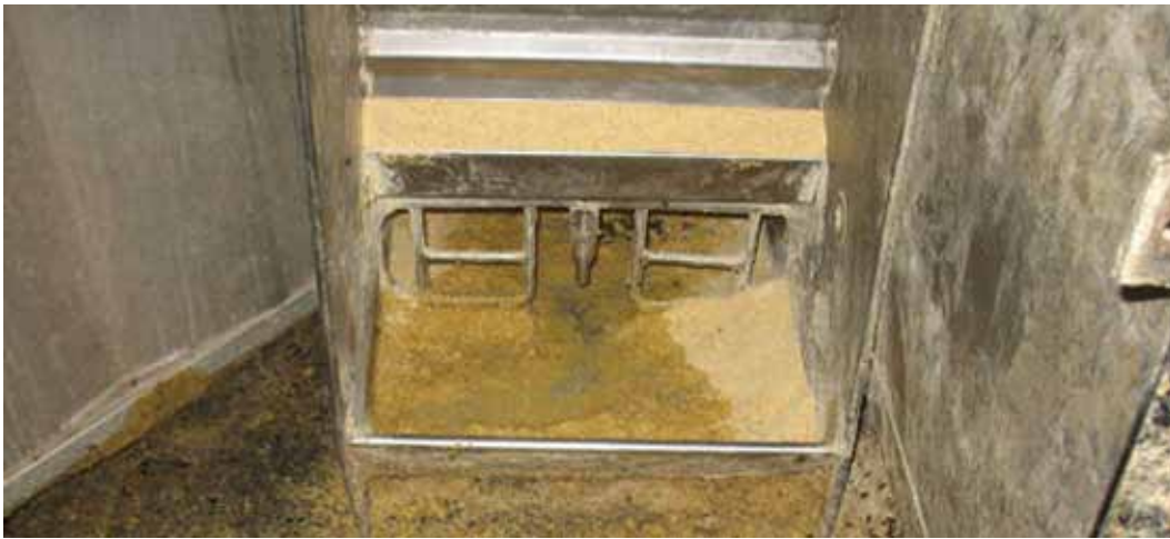
Figure 7. Wet-dry feeder at setting 18 with a 1.25-in. opening and \approx 87% pan coverage.
