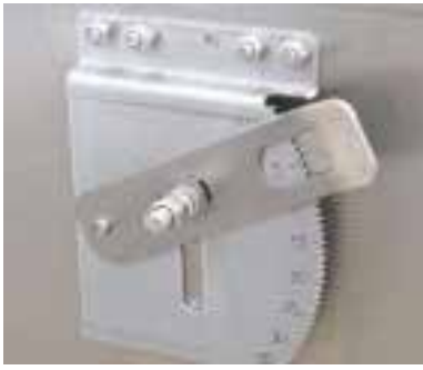
Figure 1. Feed-shelf/gap-opening adjustment mechanism located inside each end of the feed storage hopper of the wet-dry feeder.
