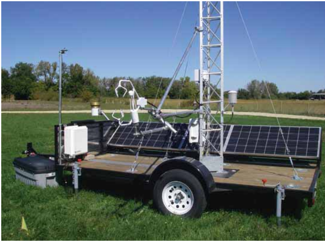
Figure 3. Trailer-mounted eddy covariance tower located at the Rocky Ford Turfgrass Research Center.
