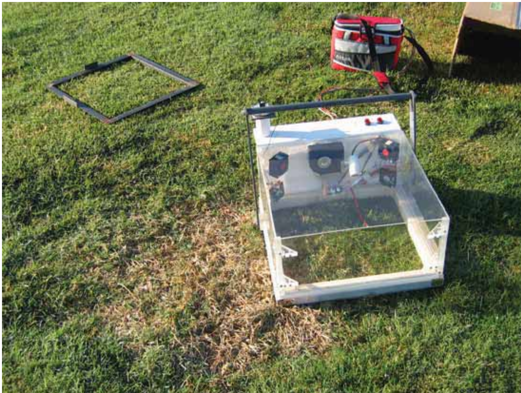
Figure 1. Large chamber fabricated to measure CO 2 fluxes in turfgrass. The system was connected to and controlled by a datalogger in the red cooler. Measurements with the sunlit chamber represented net photosynthesis of the turfgrass ecosystem.
