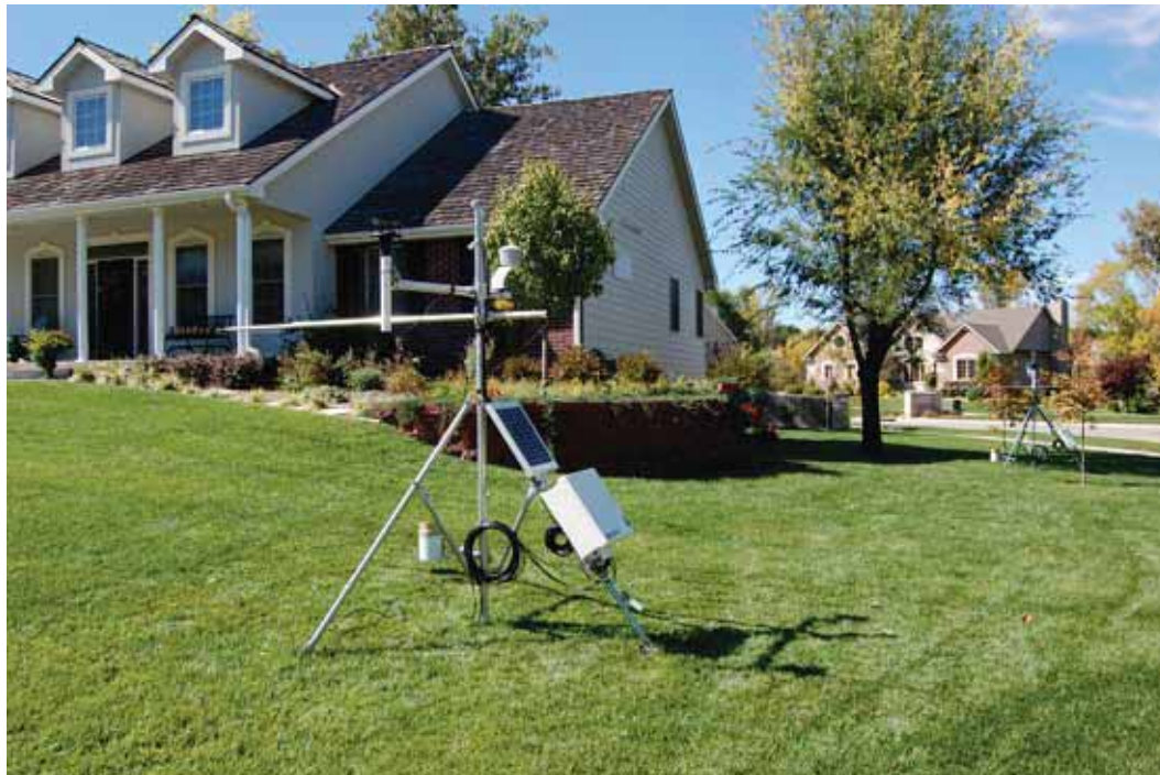
Figure 2. Two tripods deployed in a residential lawn. One sampled a relatively open area (left), and the other sampled a shady portion of the yard (right) to examine microclimates within the lawn.
