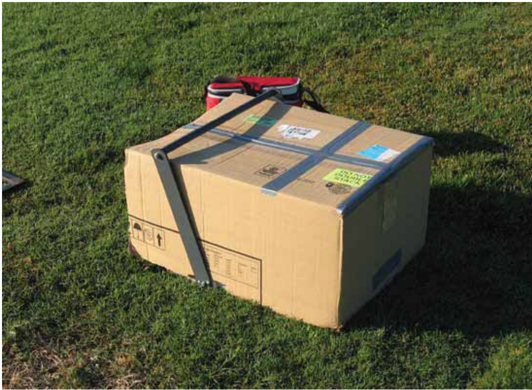
Figure 3. The chamber was shaded with an opaque, cardboard box to obtain measurements of canopy and soil respiration ( R_c + R_s ) with no photosynthesis.
