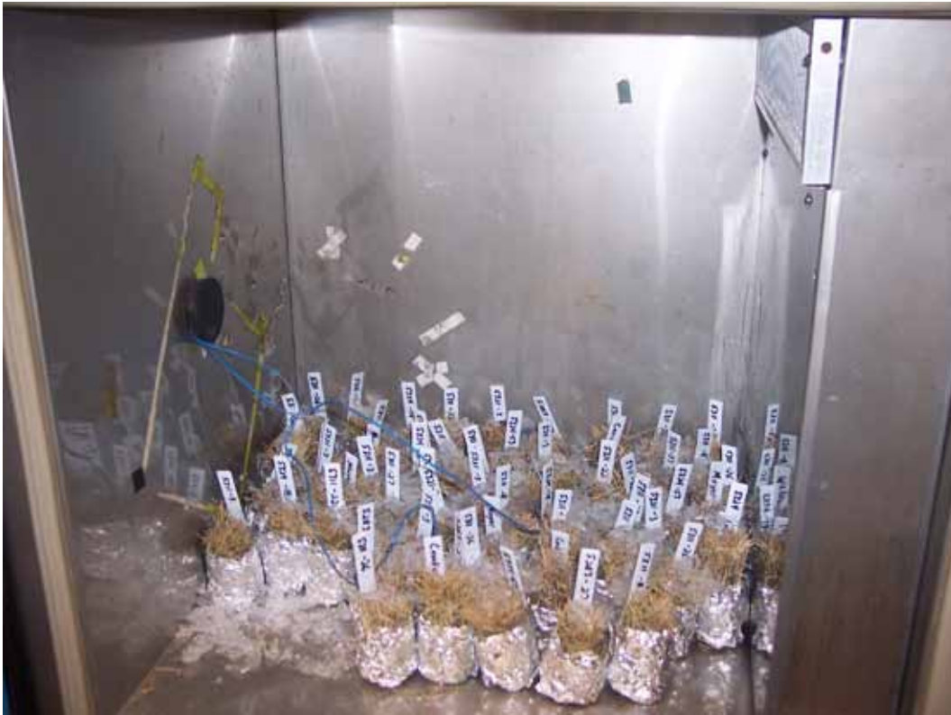
Figure 1. Plugs sampled from the field were subjected to freezing temperatures in a chamber.
