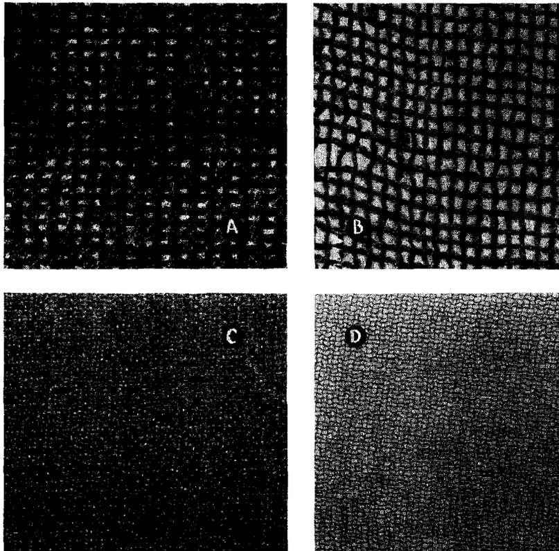
FIG. 12.—Mixed fabrics: (A) Novelty mixture of 52 percent wool and 48 percent viscose rayon. (B) Fabric A after the wool had been removed. (C) Rayon alpaca of 58 percent acetate and 42 percent viscose yarn. (D) Fabric C after the acetate rayon was removed. (Magnification 2 ×.)
