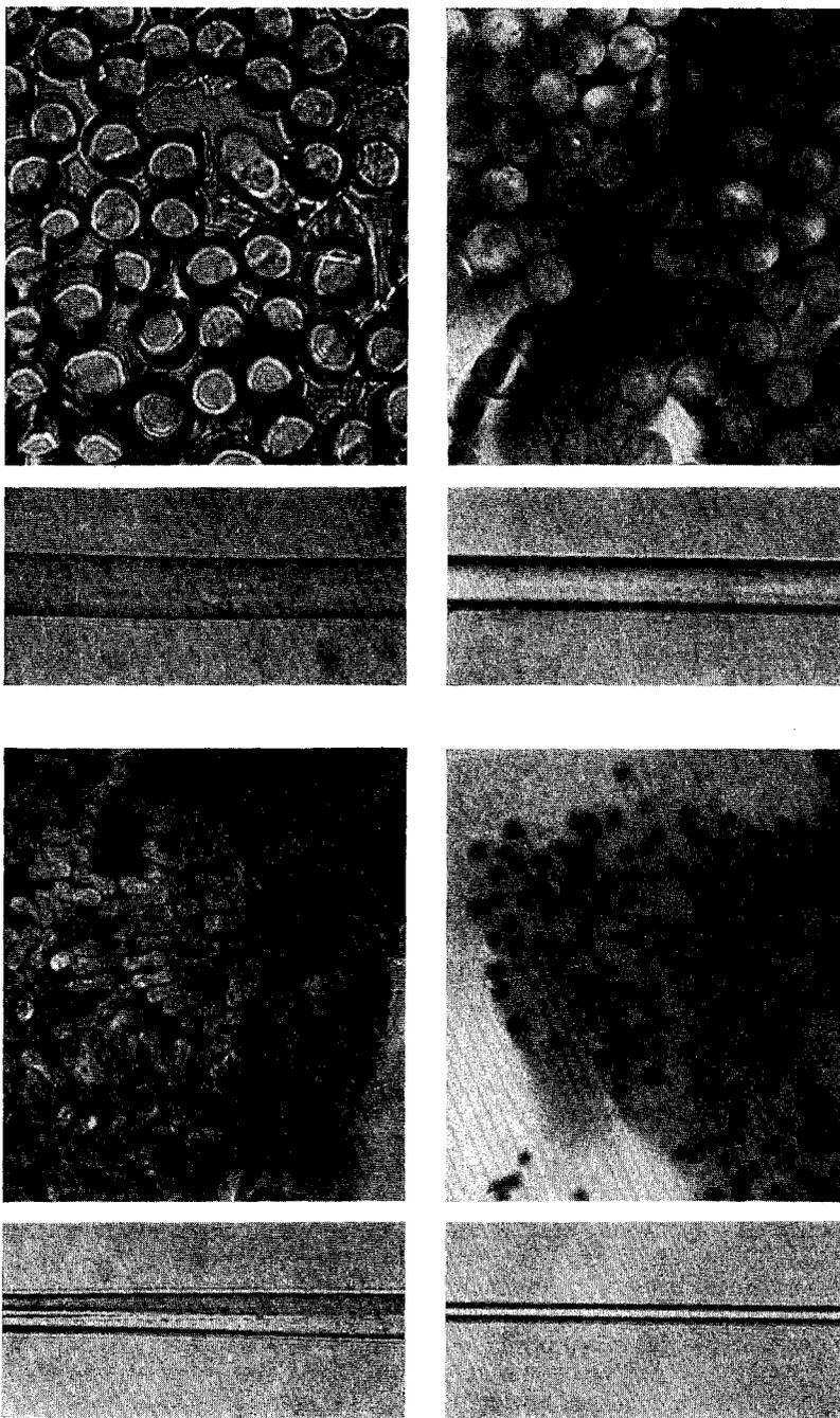
FIG. 9.—Photomicrographs of cross-section and longitudinal views of different synthetic fibers. Upper left—Soybean. Upper right—Nylon. Lower left—Vinylon. Lower right—Glass. (All magnifications 335 diameters.)
