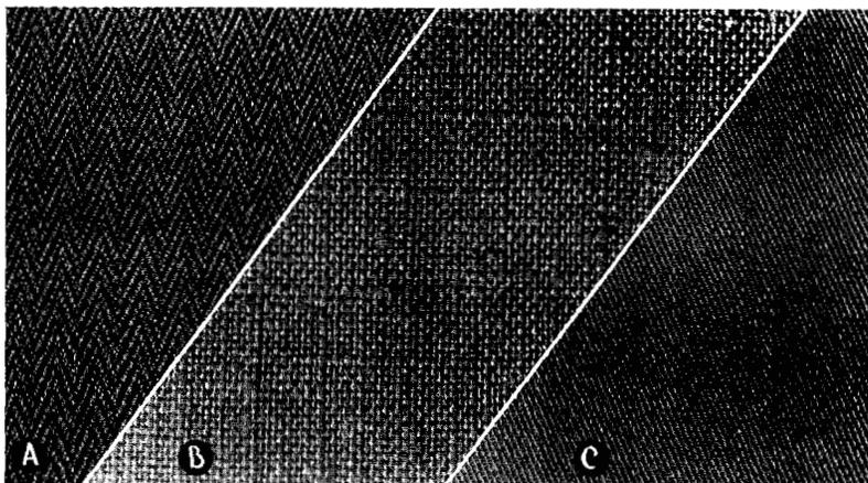
FIG. 10.—Specimens of spun rayon fabrics. A is acetate (Teca) herring-bone twill; B is viscose rayon simulating linen; and C is a viscose gabardine.
