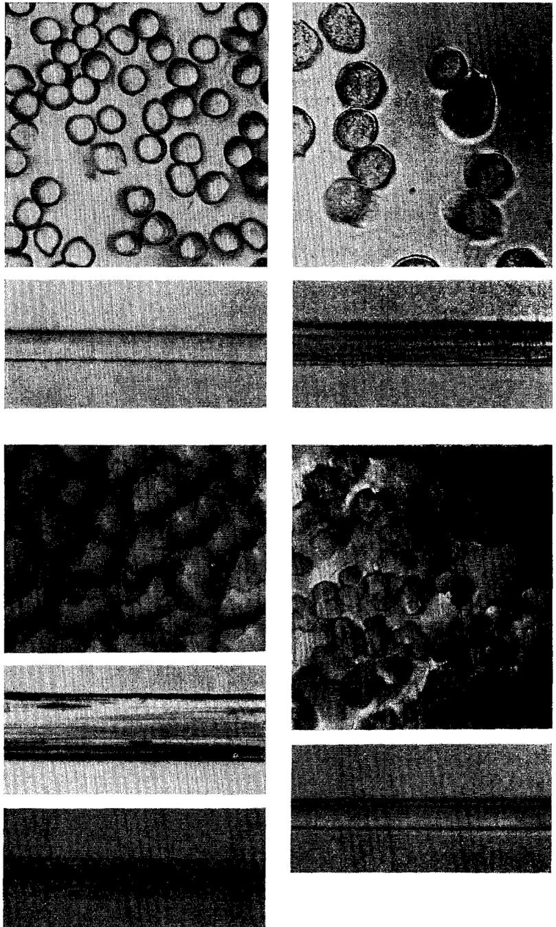
FIG. 8.—Photomicrographs of cross-section and longitudinal views of different synthetic fibers. Upper left—Cuprammonium. Upper right—Lanital. Lower left—Viscose, with longitudinal views of lustrous and delustered fibers. Lower right—Acetate. (All cross sections magnified 380 diameters. Longitudinal views 350 diameters.)
