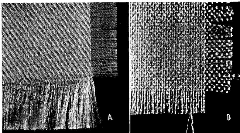
FIG. 14.—(A) Satin with silk warp and rayon filling, 55 percent cuprammonium, 45 percent silk. (B) Medium weight dress fabric of rayon and cotton ply yarns, 75 percent viscose, 25 percent cotton. (Magnification  $2\times$ .)
