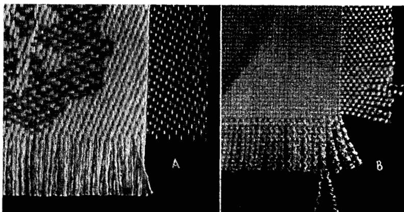
FIG. 11.—Tablecloths of viscose rayon and cotton. (A) Cotton warp and rayon filling. (B) Warp and filling of two-ply yarns, one of rayon and the other of cotton. (Magnification 2 ×.)
