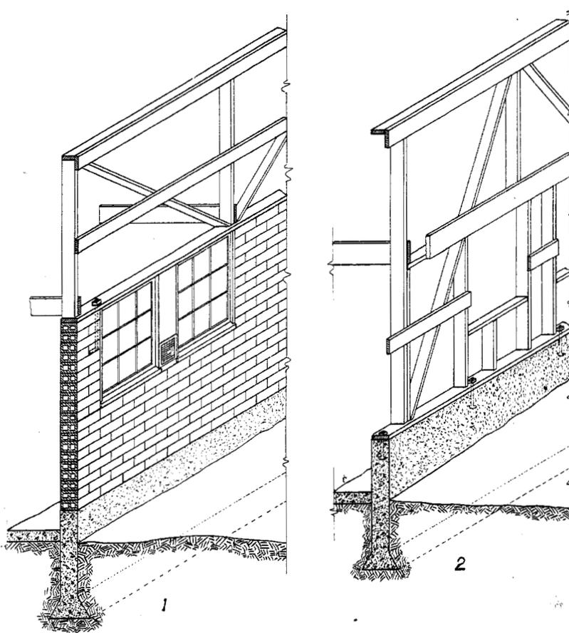
FIG. 8.—Concrete foundation with (1) tile wall and (2) frame wall.
