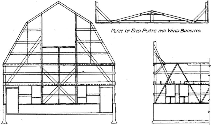
FIG. 10.—End and side wall framing and sway bracing for vertical siding.
