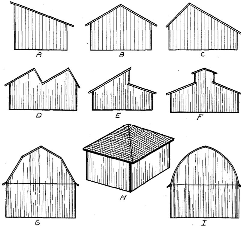
FIG. 11.—Roof shapes: (A) Shed. (B) Gable. (C) Broken gable. (D) Saw tooth. (E) Half monitor. (F) Full monitor. (G) Gambrel. (H) Hip. (I) Gothic.
