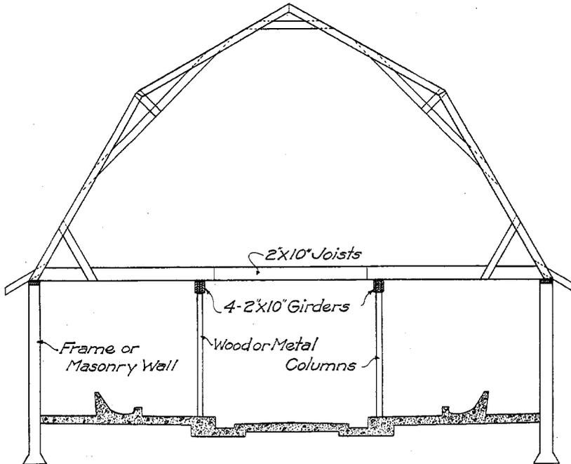
FIG. 2.—A one- and one-half-story dairy barn. This is a very practical type of barn where a large part of the necessary feed is in a silo or other building.
