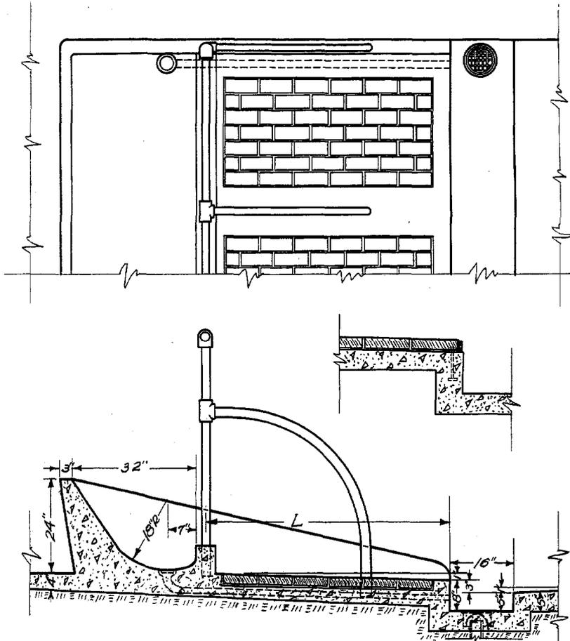
FIG. 17.—Stall plan and section, showing use of cork brick or creosoted wood-block flooring.
