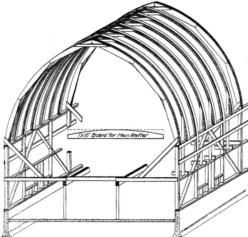
FIG. 13.—Gothic roof framing. Note the main rafter every 14 feet built up of 1" x 10" boards and sawed to curve; intermediate rafters of five 1" x 4" boards bent to radius and nailed.
