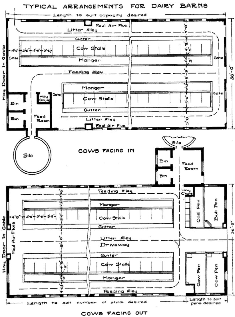
Fig. 5.—Typical floor plan arrangements for dairy barns—upper plan for cows facing in; lower plan for cows facing out.
