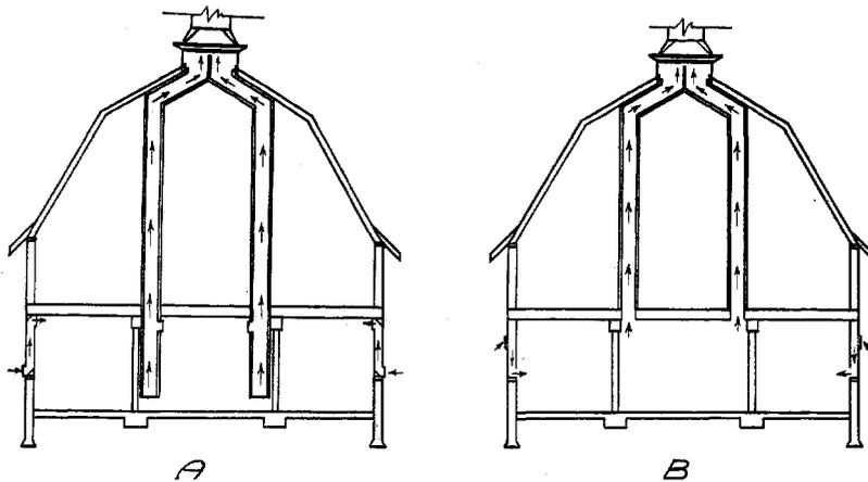
FIG. 23.—Ventilating flue arrangement. (A) The modified King system. (B) The Rutherford system. Note in A that the air enters the stable at the ceiling and foul air is removed from near the floor. In B fresh air enters near the floor and foul air is taken out at the ceiling. The modified King system has a small opening in the flue near the ceiling.
