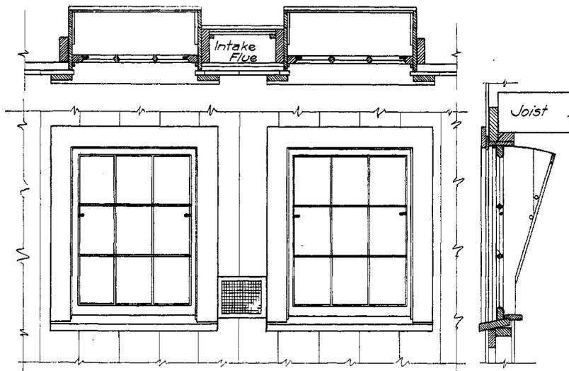
FIG. 22.—Nine-light windows, placed in pairs with intake ventilating flue between, is a very popular installation. Note the ventilating shield which deflects the air toward the ceiling when the window is tilted inward at the top, preventing direct draft on the cows. The window may be raised a few inches when in the open position so as to allow a direct draft for summer.
