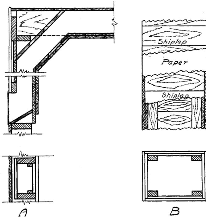
FIG. 24.—Details of ventilating flue construction. (A) Intake flue.
