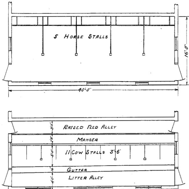
FIG. 38.—Remodeling suggestion. An unused stable may be converted into a well-arranged dairy section. Posts may have to be moved latterly to conform to new stall widths, but this shift usually can be made if an additional piece is added over the posts. Extra windows must be added, which can be done without disturbing those already in place.
