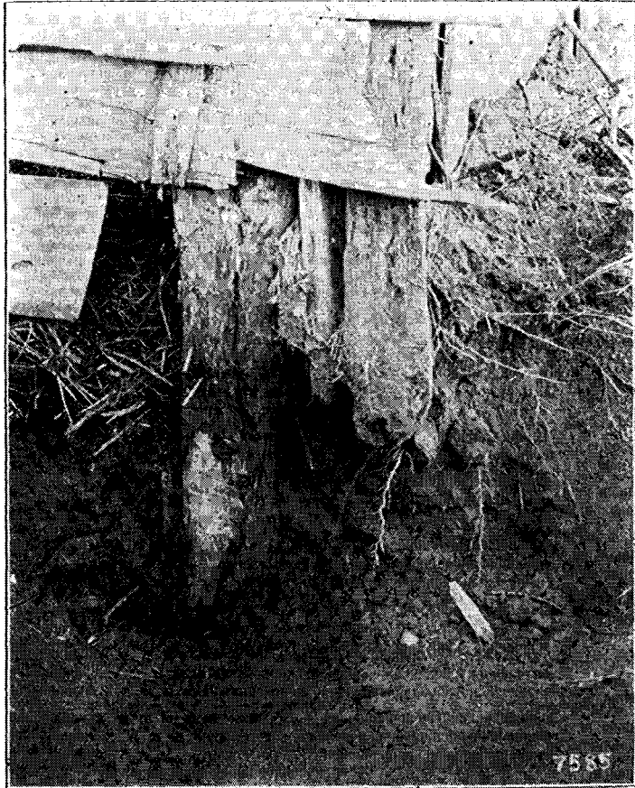
Plate 37. From photograph furnished by United States Bureau of Forestry. Post from timber of Catalpa speciosa Ward, five or six years old, in ground for fifteen years. Note sound character of the wood shown in the cut face, to the left at the base of the post.
