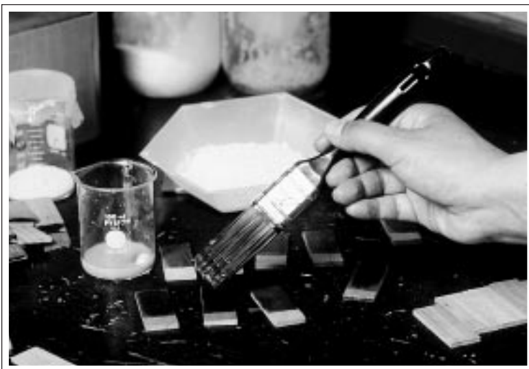
An adhesive made from soybeans has good strength and water resistance.
