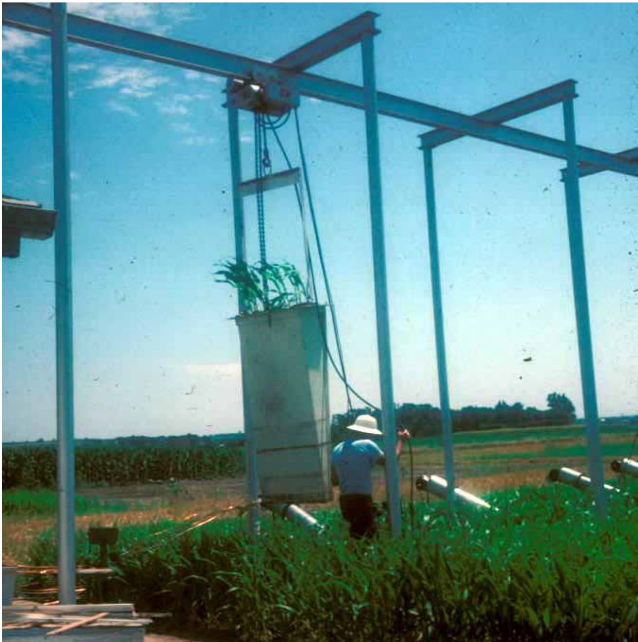
Rhizotron with glass-sided chambers for researching root growth, 1984.
