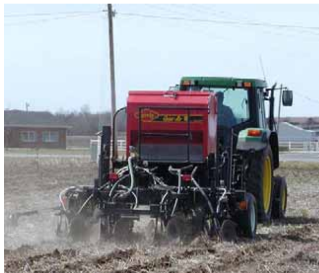
Machine for strip tillage and fertilizer placement before planting corn, East Central Experiment Field, 2003.
