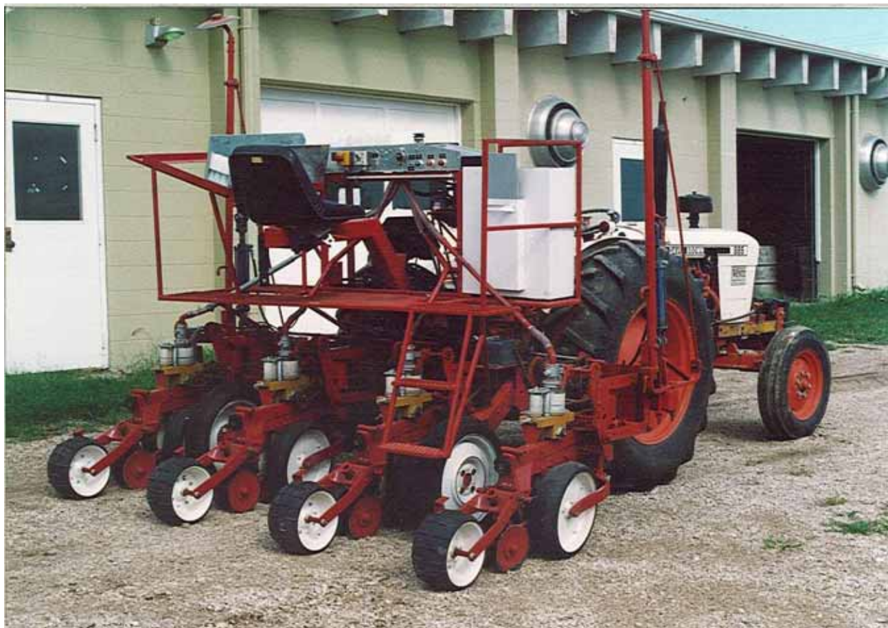
Plot planter designed by Clarence Swallow and constructed in the Agronomy Farm shop, 1987.
