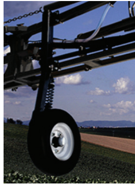
Figure 2. Gauge wheels measure pressure between the wheel and the ground to determine boom height.
