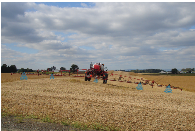
Figure 3. Ultrasonic sensors on ABHC technology monitors boom height at a various locations to maintain uniform boom height.
