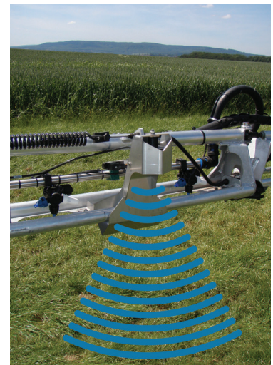
Figure 1. Ultrasonic sensor mounted on the sprayer boom.
