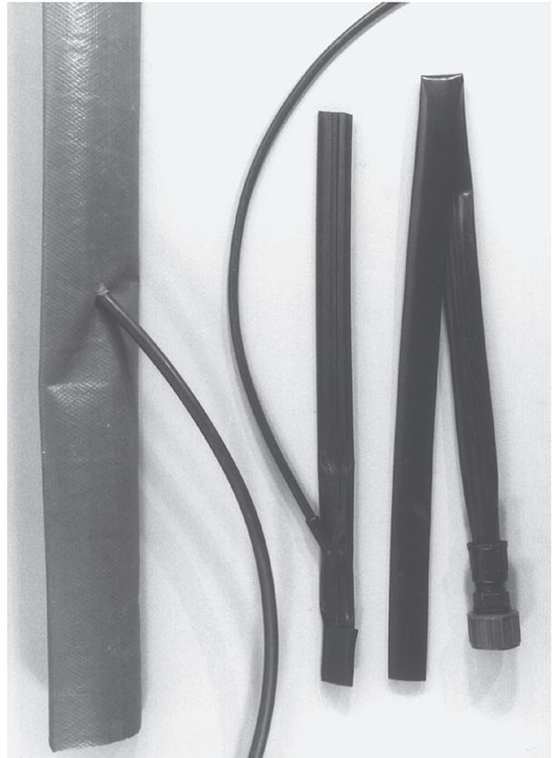
Vinyl lay flat hose with feeder tube attached (left), Feeder tube inserted into drip tape (center), and plastic drip tape (right).
