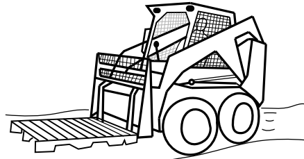
Driving on level ground with the attachment low.
